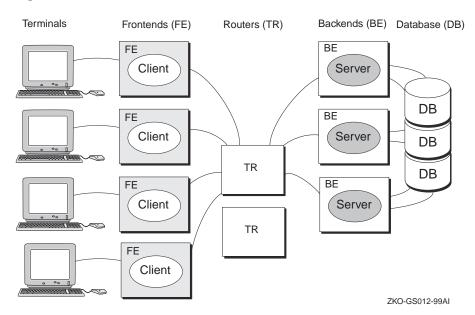
Figure 2–2 Partitioned Data Model
